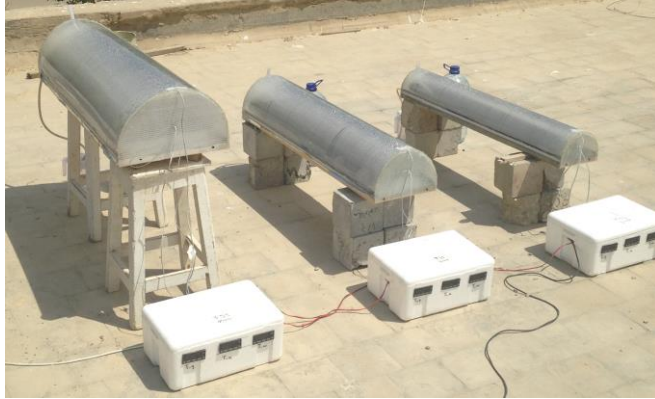
Fig. 3.6 Experimental set-up of the half-TSS model with variable tray dimensions
