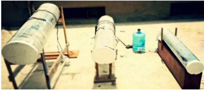
Fig. 3.4 Experimental set-up of the full-TSS model with constant tray dimensions
