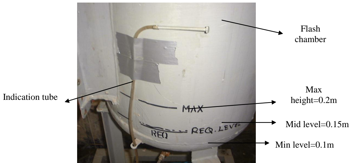
Figure (6.19) The position of the level indicator tube
