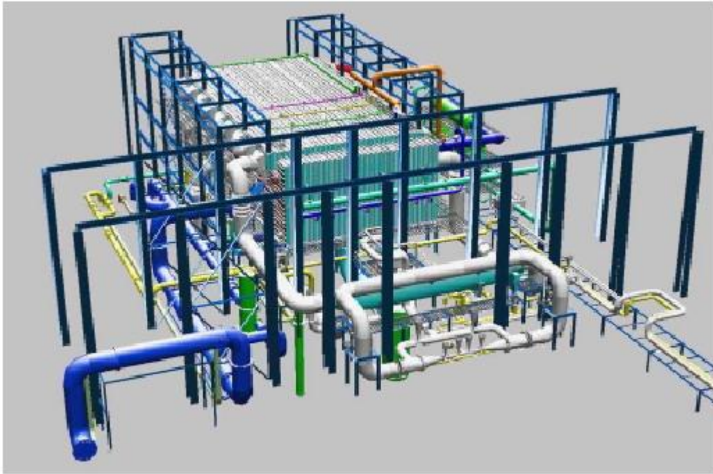
Figure (2.12) shows a schematic diagram of a real MSF plant [11]
