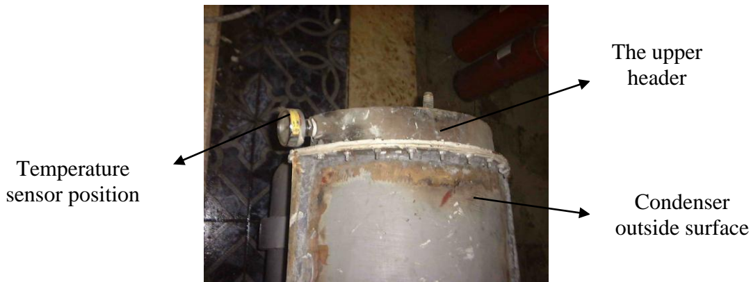
Figure (6.16) The position of the temperature sensor that measure the preheated feed temperature
