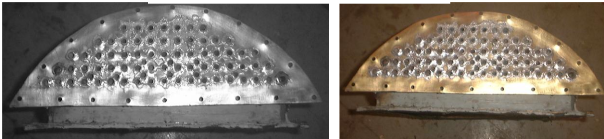
Figure (6.10) The distribution of the tubes at the upper side from the condenser
