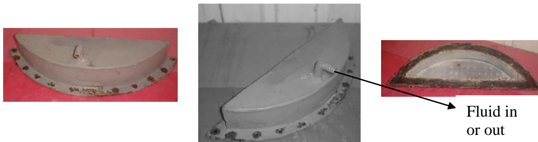
Figure (6.12) The photograph of different views of the upper and lower covers of the headers of the condenser
