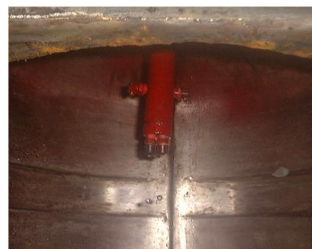
Figure (6.8) The photograph of the injector inside the flash chamber
