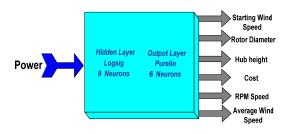
Fig 3: HWT Neural Network Model concept.
