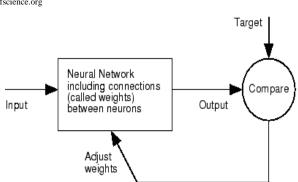
Fig 2: Schematic diagram of ANN concept.
