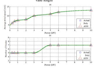
Fig 8: Data results comparisons for VWT based on (a) average wind speed, (b) number of blades.
